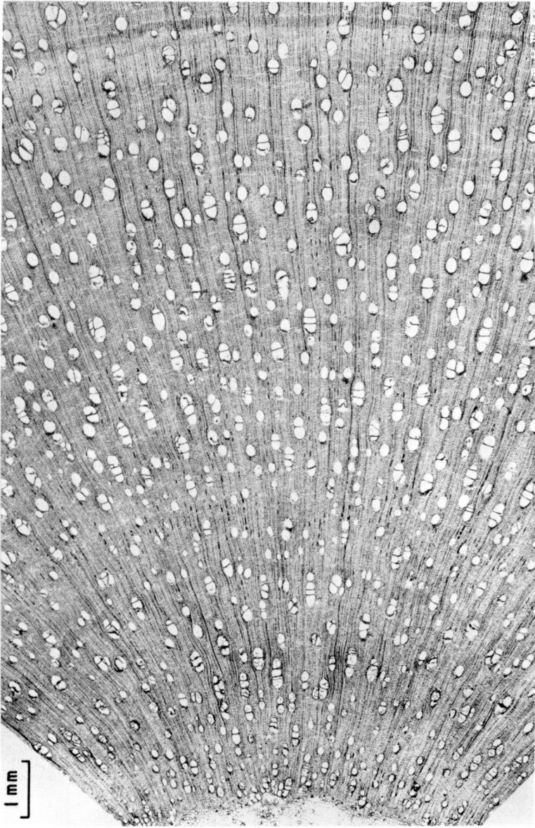
Figure 43. Cross section through sapwood of mature tree. \times 10 .
