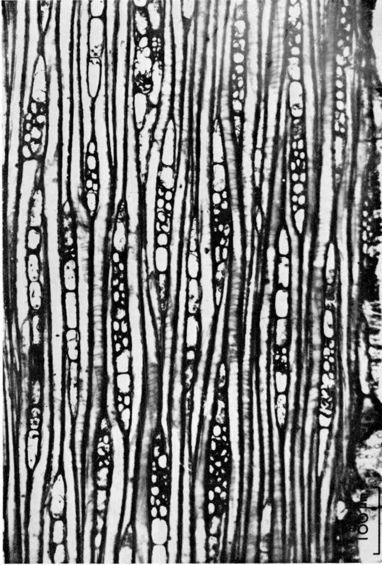
Figure 44. Tangential section through sapwood of a mature tree. × 170.
