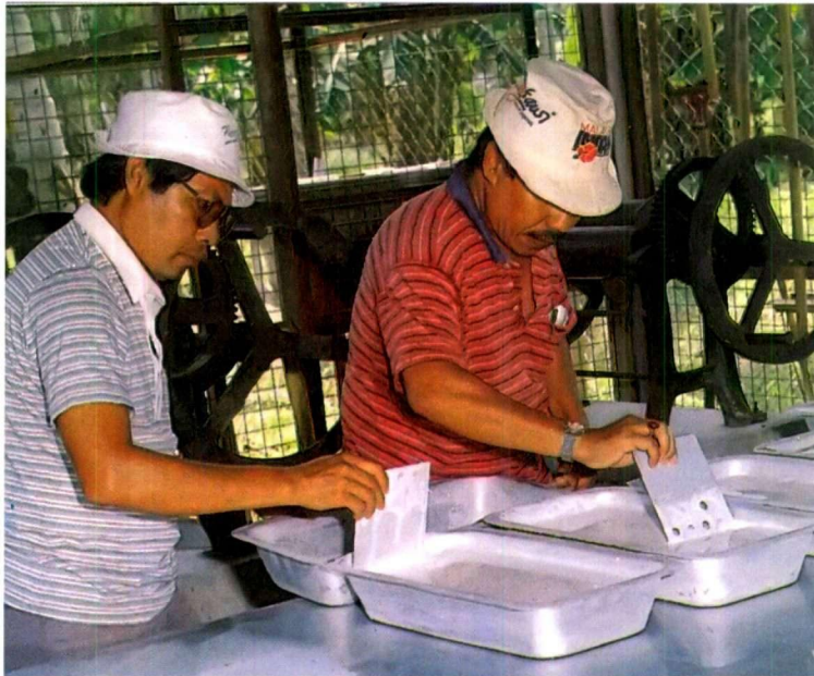
(a) Gentle stirring to mix acid and latex in pans for coagulation
