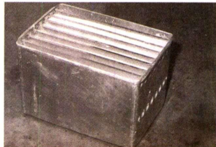
(f) Placing partition plates
