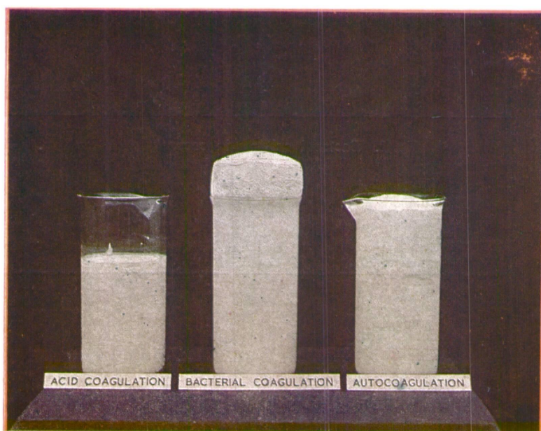
Fig. 4. Physical appearance and blown-up nature of bacteria-coagulated rubber.
