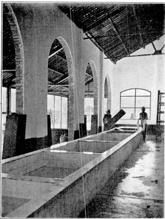
ANOTHER BATTERY OF TANKS, WITHOUT DILUTION TANKS OR MEANS OF GRAVITATING LATEX.
