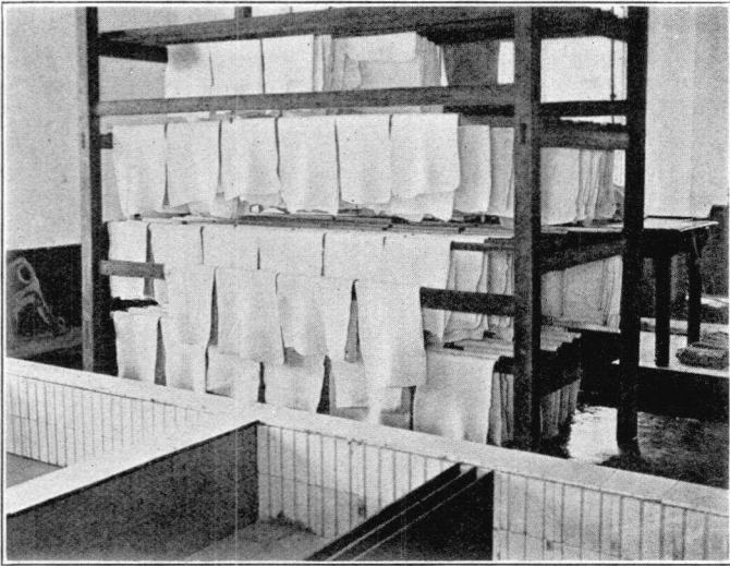
THE OLD METHOD OF "DRIPPING" FRESHLY ROLLED SHEETS WITHIN THE FACTORY.
