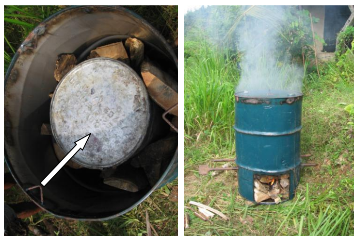
Fig. 1. Small scale biochar production: A biomass filled, closed, small vessel is placed inside a large barrel (left) and then cooked (right)
